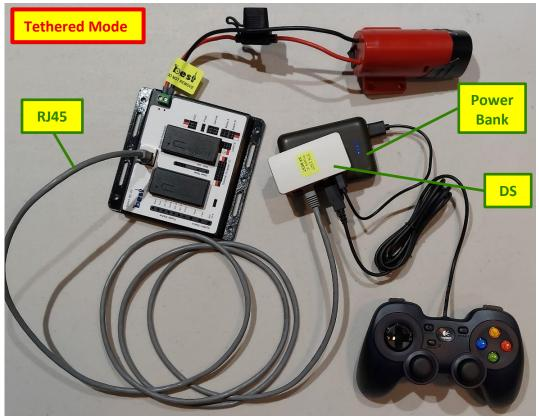
**Power Bank (w/ USB-micro charge cable)** – provides power for the driver station and Joystick. Recharge with the included USB-micro charge cable.
