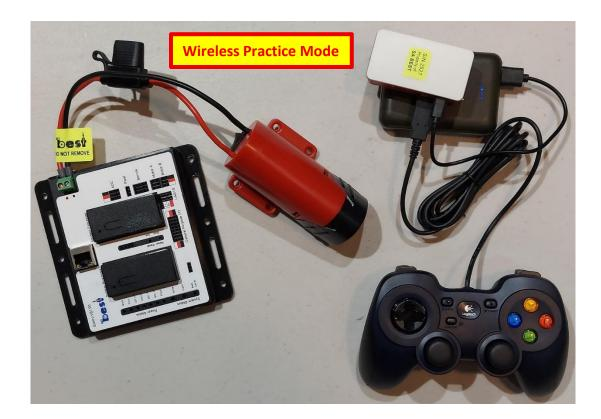
**Binding:** The Gizmo and DS must be properly "bound" for the communications to work. Team Gizmo/DS were bound prior to distribution, and the most reliable method is described below.
