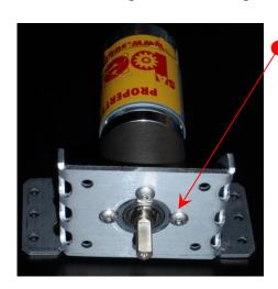
These motor mounting screws use the 3/32" Allen Wrench included in return kit.
